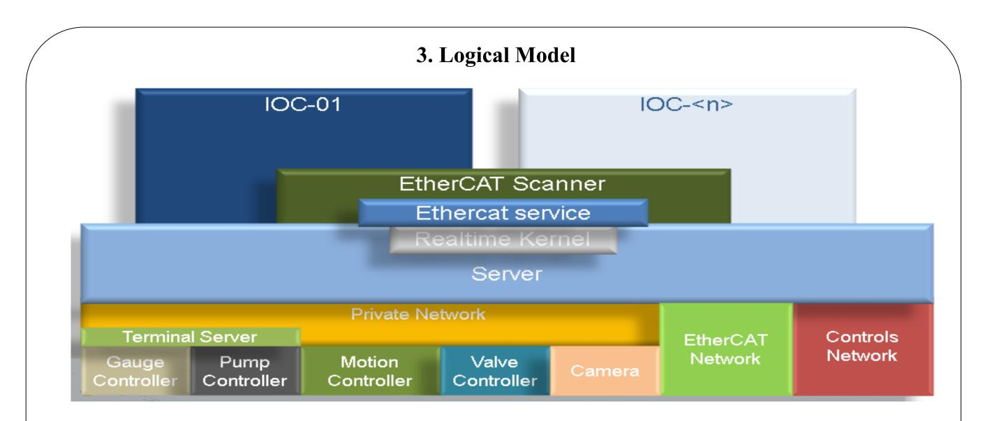
This diagram provides a logical representation of the Linux server in context with the I/O subsystems, traversing upwards to one or more EPICS IOC instances. The Linux PCs are standard Dell 1U discless servers (currently R320), that boot from an image over the network into a RAM based disk.
