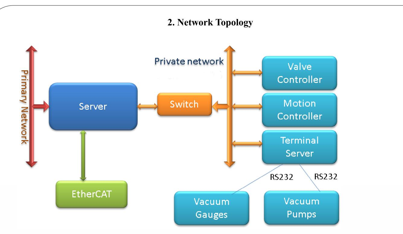
The servers are supplied with four network interfaces. This is to facilitate multiple dedicated and isolated networks, typically three are used as:
