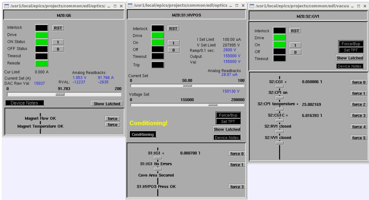
Figure 4: Visualization of interlocks for M20 optical and vacuum devices.
