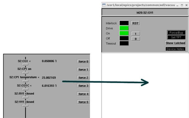
Figure 2: Interlock panel (on the left) is embedded in lower part of control device panel (on the right).
