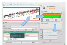
Figure 3: example of widget interactivity, selection of an active alarm will highlight in red the related devices in the Synoptic, where they can be selected for the Device panel or dragged into the Taurus trend.
