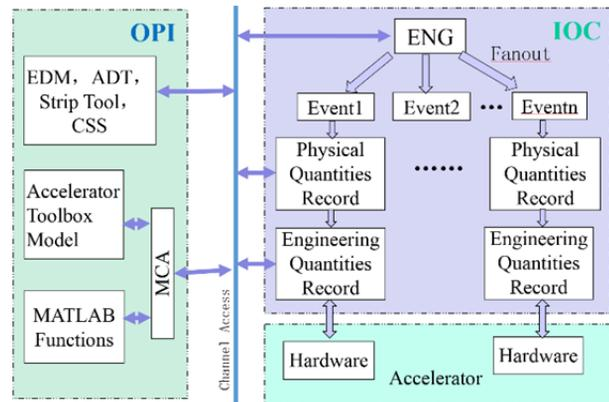
Figure 1: Functional diagram of the HLS-II control system.
