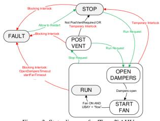
Figure 3: State diagram for 'Type 2' AHU
