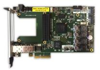
Figure 3: Simple PCIe FMC carrier (SPEC).
