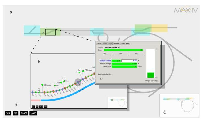
Figure 2: Synoptic for the linear accellerator of MAX IV. Initially an overview of the entire machine is shown (a). The user can zoom in on a particular region (b) to reveal individual equipment such as magnets. To access a particular device, a specific GUI (c) can be opened. A "thumbnail" (d) shows the current view in relation to the whole. A row of buttons (e) allow the user to control the visibility of individual subsystems.
