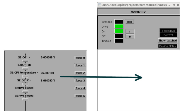
Figure 2: Interlock panel (on the left) is embedded in lower part of control device panel (on the right).
