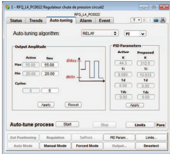
Figure 2: UNICOS auto-tuning user interface: Relay method.
