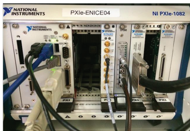
Figure 1: The GMT module installed in slot 5 of a PXI Express crate.
