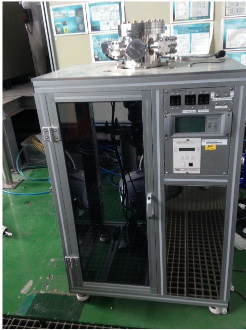
Figure 4: Demo vacuum control system with turbo pump and several vacuum gauges.
