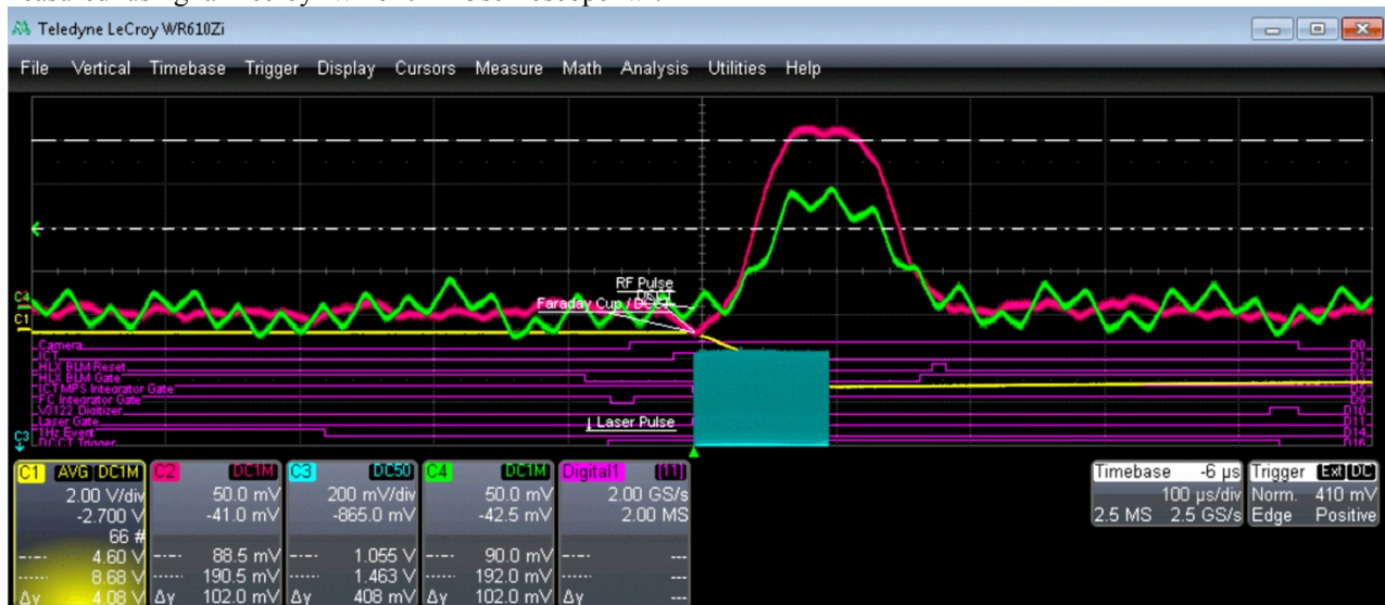
Figure 3: ERL accelerator instrumentation with the laser gate on a digital multiplexed oscilloscope.
