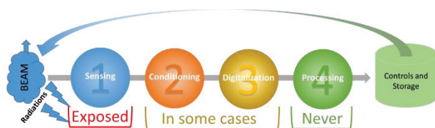
Figure 1: Typical structure of an instrumentation acquisition system. The signal from the sensor is conditioned, digitized and in line processed.
