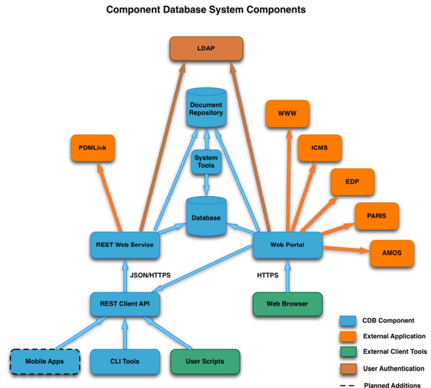
Figure 1: CDB system architecture. Dashed lines indicate future components.
