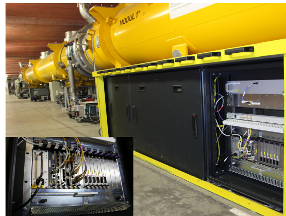
Figure 1: Installation of MicroTCA crates inside the FLASH tunnel underneath the accelerator module. The radiation shielding (yellow cabinet) protects the electronic rack inside. The insert shows the MicroTCA crate installed in this rack.
