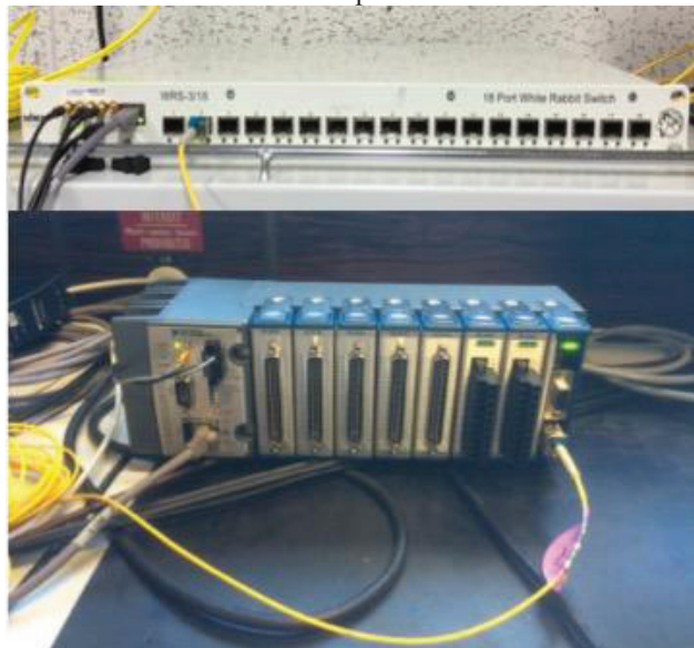
Figure 2: The test setup with the cRIO-WR module connected with the yellow fibre to the WR switch on top.
