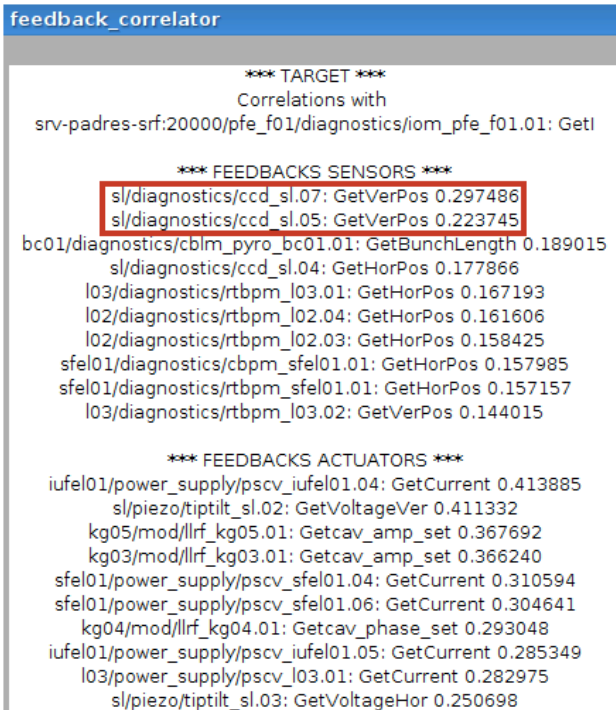
Figure 3: List of sensors/actuators most correlated with the FEL intensity; seed laser vertical positions on the two CCDs on top of the ranking indicate a seed laser transverse misalignment.
