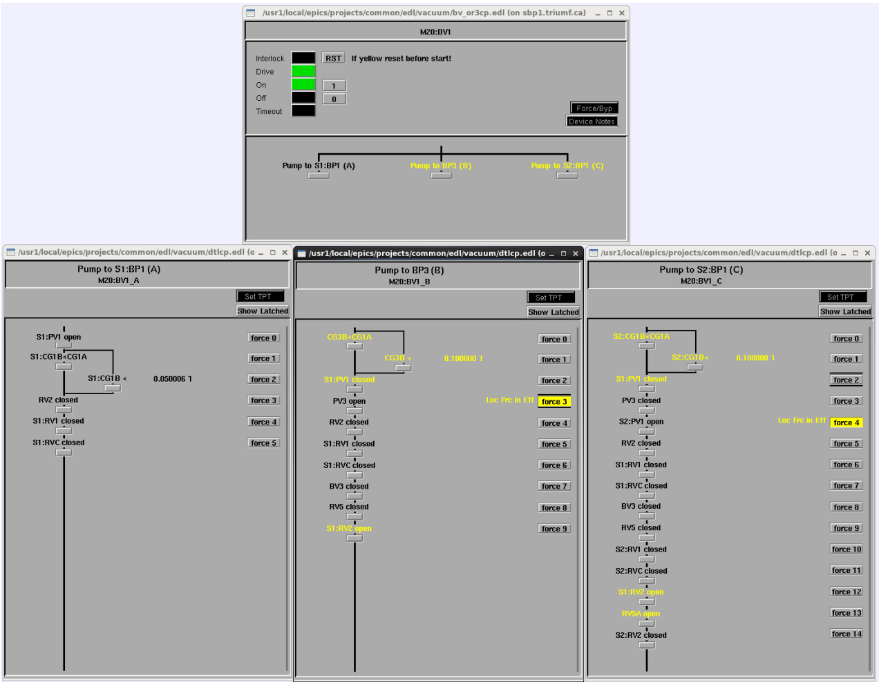
Figure 3: Example of hierarchical interlock chains implemented for M20 Secondary Beam Line.
