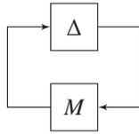
Figure 2:  $M$ - $\Delta$  structure for robust stability analysis.
