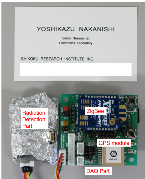
Figure 1: A prototype KURAMA-micro unit. The board on the right is the DAQ part based on OpenATOMS architecture. The left part shielded by aluminum foil is the radiation detection part. Both are implemented into a box of business card size. The power required for the unit is managed by a 3.7 V rechargeable Li-ion battery.
