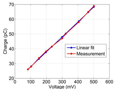
Figure 5: Characteristic of the bunch charge detection subsystem.
