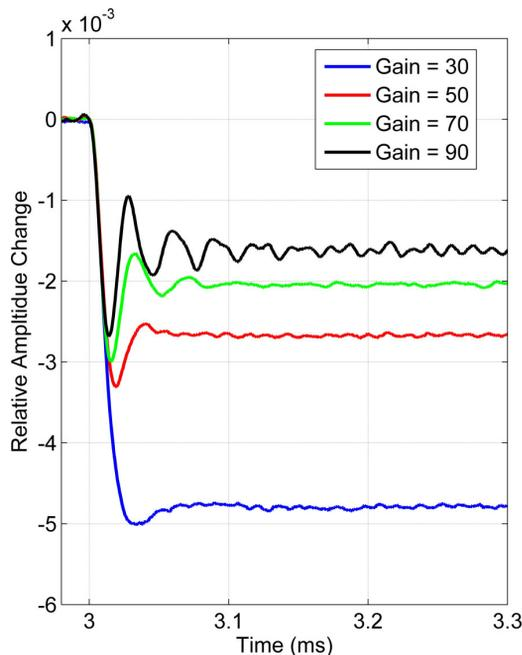
Figure 2: Response of a LLRF system using only a PI feedback controller to a beam pulse (zoom in during beam rise).
