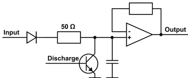
Figure 3: Block diagram of the peak detector.
