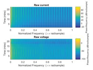
Figure 2: Spectrograms of voltage and current signals
