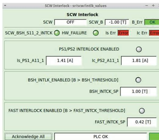
Figure 6: The SCW interlock GUI.
