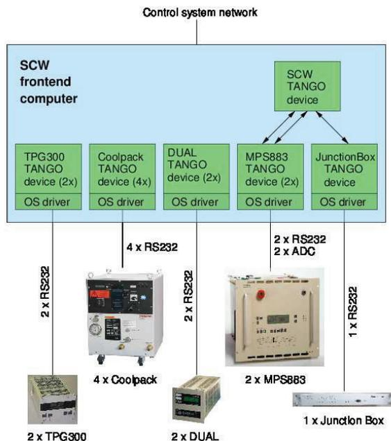
Figure 4: TANGO device servers layout on SCW front-end computer.
