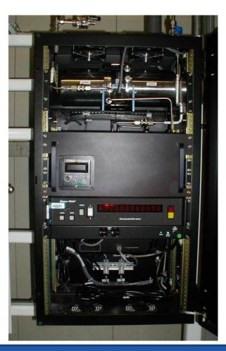
Femto-TECH Model GC224RM gamma-compensated ion chamber
