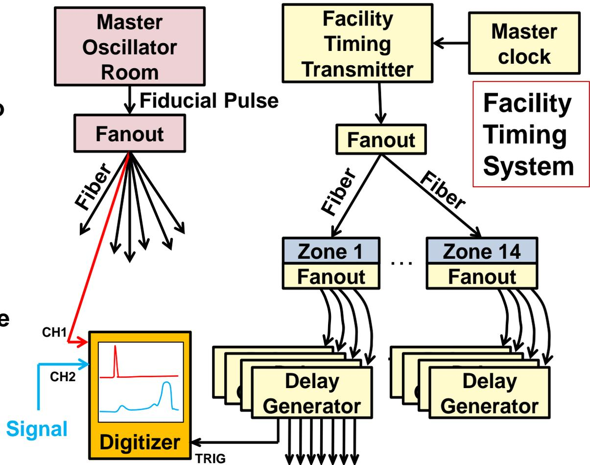
The ITS controls hundreds of devices, and the fiducial provides a precise, stable reference for timing measurements.
