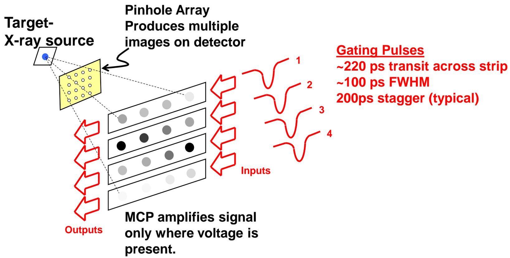
There are a variety of gated x-ray detectors in use at the NIF. Results here are for CCD-based GXD's, but other diagnostics perform similarly.
