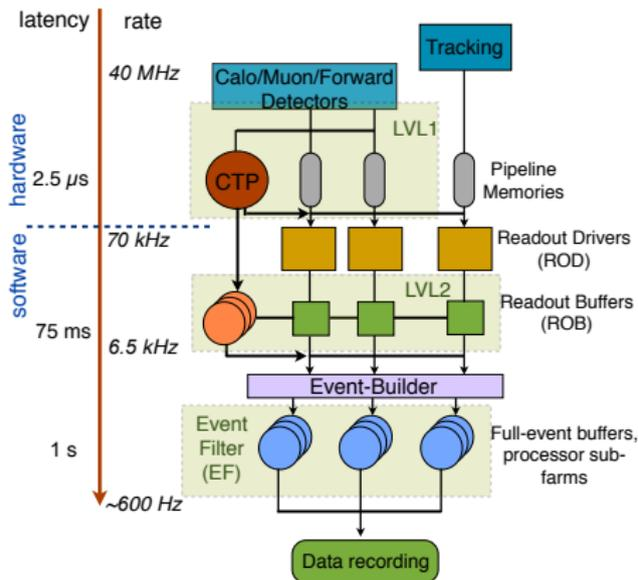
Typical rates for Run I above. Expected in Run II: 100 kHz L1, 1 kHz HLT.
