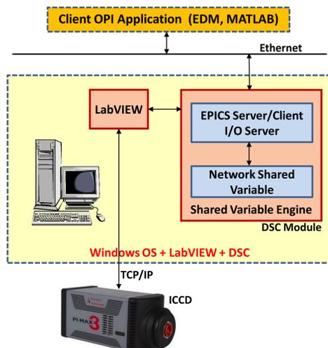
Fig 2. Infrastructures for the Intensified CCD camera.
