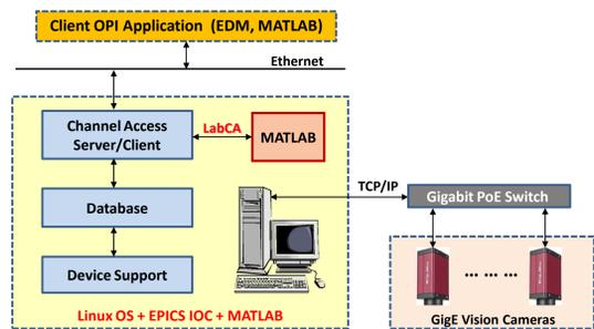
Fig 1. Infrastructures for the screen monitor CCD camera.
