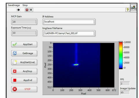
Fig 7. LabVIEW control/display GUI for ICCD.
