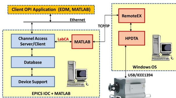
Fig 3. Infrastructures for the streak camera.
