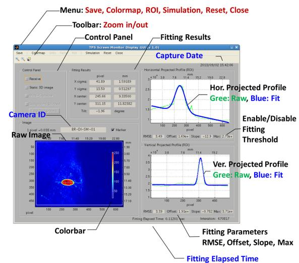
Fig 5. Matlab analysis display GUI for screen monitor.
