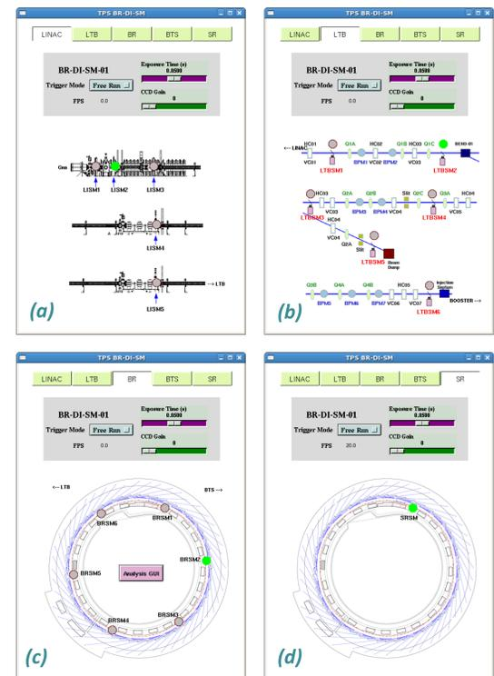
Fig 4. The EDM camera control user interfaces for the screen monitor of (a) Linac, (b) LTB, (c) BR, and (d) SR. The top bar can switch in between the five pages, and the cameras location shows in below.
