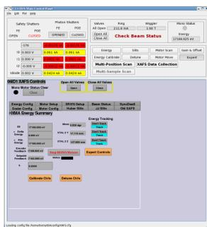
IDA at the HXMA beamline. This screen shot was taken when the beamline was inactive, causing the “Check Beam Status” message. The red and yellow boxes in the upper left are read-backs from different detectors, the coloring intended to warn the user when data being collected is outside the optimal range. In the lower part of the screen, an embedded EDM window saves on re-development effort.
