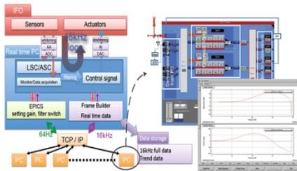
Figure: The design concept of the KAGRA digital system
