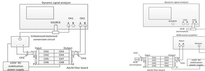
Figure: Block diagram of inspection of AA/AI filter board performance. Left figure is Evaluation of the transfer function of LPF and SNF filter signal performance. Right figure is Measurement of equivalent input noise.
