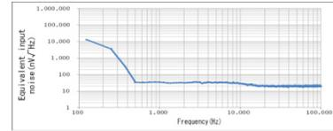
Graph: Sno.1 CH1 Measurement of equivalent input noise (scope of 0-10kHz)
