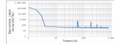
Graph: Sno.1 Measurement of equivalent input noise (scope of 0-1kHz)
