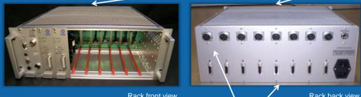
EMC-shielded connectors for motor and encoders
