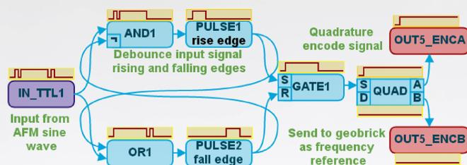
The AFM outputs a 0 - 5 V sine wave that corresponds to its scanning frequency (IN\_TTL1). ZEBRA uses two pulse generators, two logic gates, and a set-reset gate to debounce the signal, before quadrature encoding it. It is output as a differential quadrature signal to a motion controller (OUT5\_ENCA and ENCB) to use as a speed reference.
