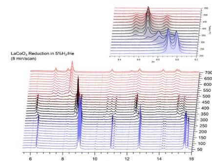
HRPD: consecutive short scans (8 min) allows to resolve sharp diffraction peaks while changing the sample environment
