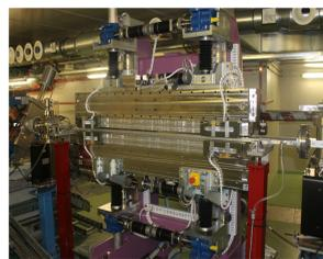
ID (undulator) located in the accelerator's tunnel
