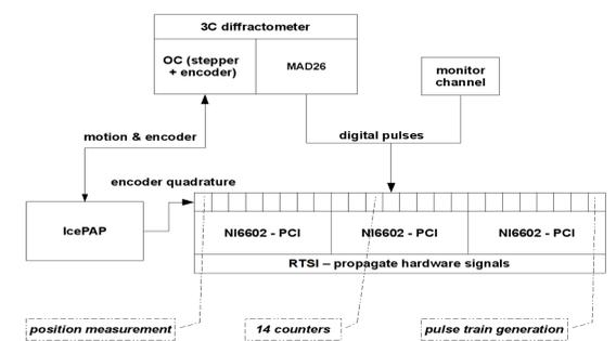
Instruments and controls hardware involved in HRPD experiment
