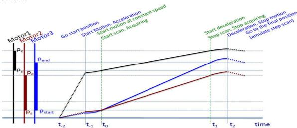
Theoretical trajectories of motors involved in the continuous scan: constant velocity represent an "effective" scan region.
