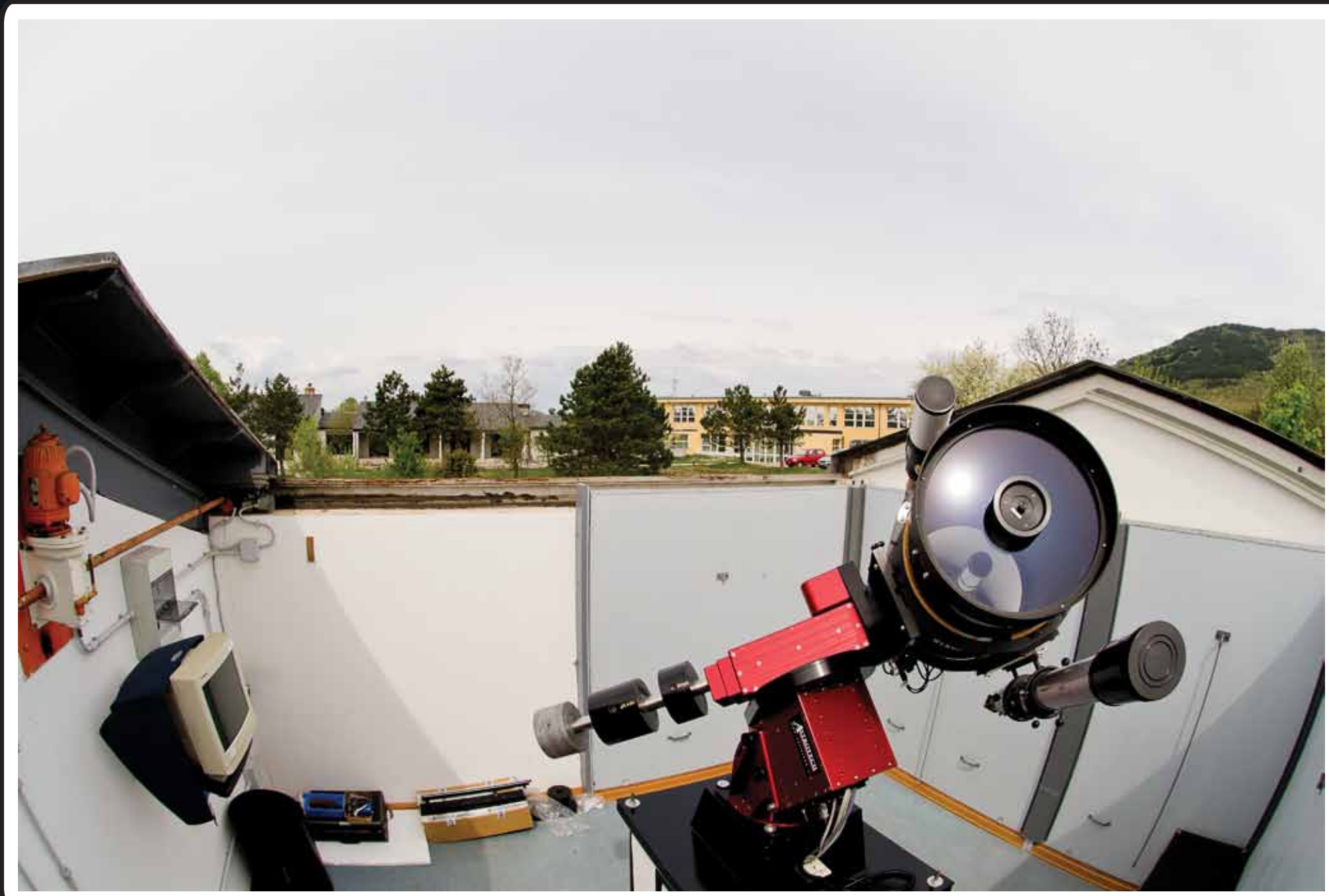
Figure 1: Telescope Celestron C14 and the solar telescope Coronado HELIOS on the Paramount ME mount, at the Astronomical Observatory of Basovizza
