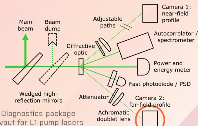
Diagnostics package layout for L1 pump lasers
