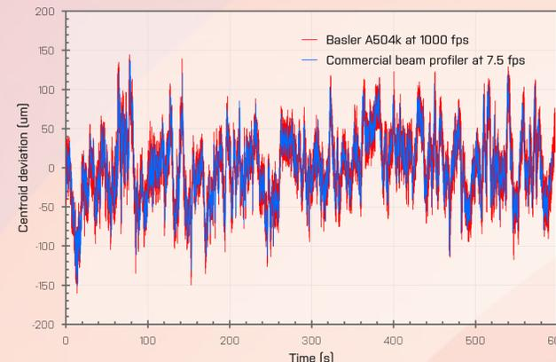
Measurements of beam centroid are precise and consistent. At 1 kHz this information can also be used for pointing stabilisation, eliminating the need for additional sensors
