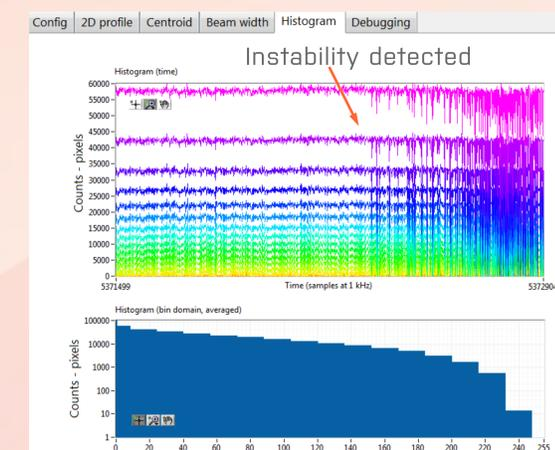
System front panel. Real-time histogram analysis gives early warning of amplifier instability that might be masked in measurements of pulse energy alone
