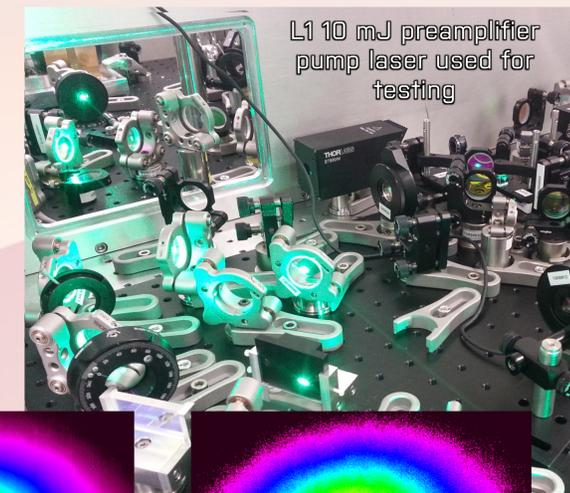
L1 10 mJ preamplifier pump laser used for testing
