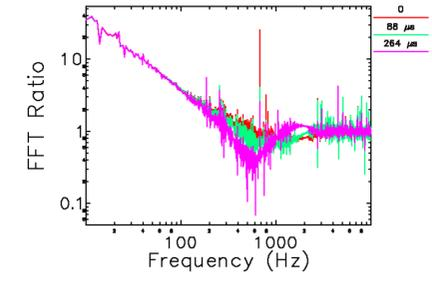
Figure 5 The FFT ratio of the raw v.s corrected orbit of APS horizontal S10A:P2 BPMs at different delays.
