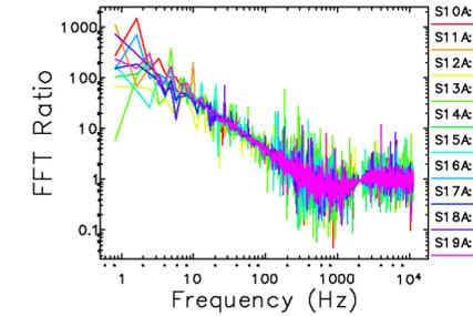
Figure 4 The FFT ratio of the raw v.s corrected orbit at some APS A:P2 BPMs using feedback configuration of 78 corr. And 78 BPMs
