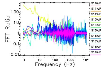
Figure 3 The FFT ratio of the raw v.s corrected orbit at some APS A:P2 BPMs using feedback configuration of one corrector (S12A:H3) and one BPM (S12A:P2).
