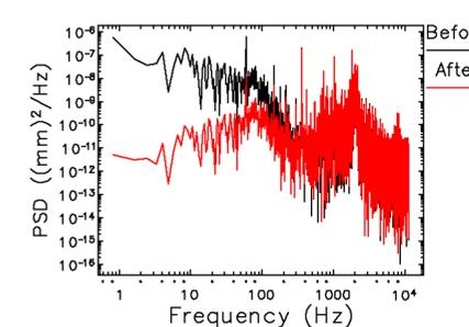
Figure 6 The PSD of APS horizontal S10A:P1 BPM before and after feedback correction.
