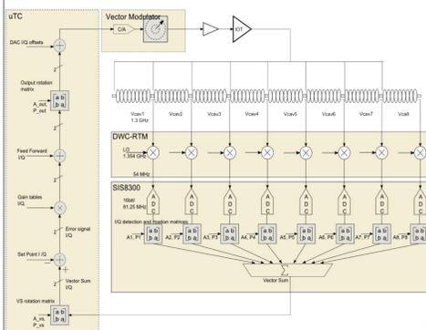
The system consists of MTCA.4 hardware components for data acquisition fast feedback loops realization, cavities signals down-conversion, drive signal up-conversion, piezo driver communication and others.
