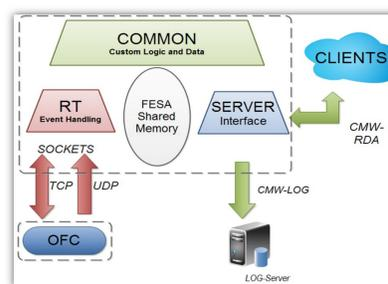
Software interfaces implemented by the OFSU server. The next FESA framework released is presently being investigated offering access to the new CMW middleware (RDA3 based on ZeroMQ) provided by CERN-BE/CO as an alternative to the present RDA2 (CORBA-based)
