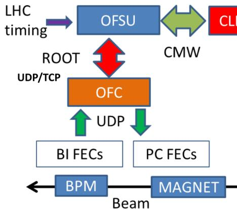
Slowly changing parameters and acquisitions typically updated at 1Hz are handled by the service-unit (OFSU) server over CMW (RDA2). The OFSU also triggers optics and critical reference orbit changes (~10 changes / cycle).
