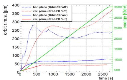
The orbit feedback is essential for LHC operation with high intensity as the required stability cannot be obtained by feed-forward alone. Its performance is better than initially specified.
