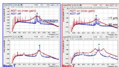
The performance of the LHC tune feedback is limited by the quality of the tune signal. With high beam intensity, the transverse feedback (ADT) as well as non-linear fields strongly degrade the signal quality.
