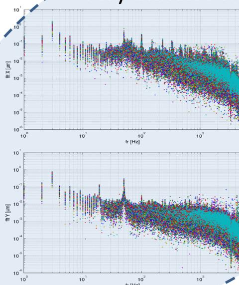
The aluminium vacuum chamber acts as a low-pass filter with pole around 200Hz.
