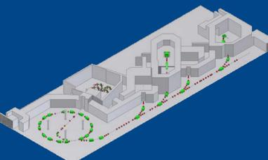
The MedAustron accelerator, featuring four ion sources, IH-based Linac, synchrotron, three horizontal, one vertical beam line and one proton gantry. Energy ranges from 60 to 800 MeV/u, up to 250 MeV/u proton equivalent for ion therapy [2].
