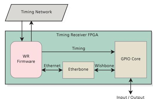
Figure 3: This is a simplification of the designed timing receiver architecture. It shows how the White Rabbit firmware interfaces are connected and what kind of data is being exchanged. Everything except the WR firmware is considered to be custom. The wishbone bus is used for accessing registers in the GPIO Core.
