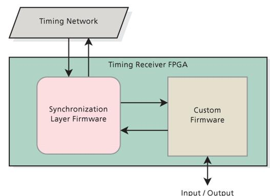
Figure 2: The timing receiver firmware can be seen as two separate modules. The synchronization layer, which is given by the vendor (MRF/WR), and the custom part, which is implemented as part of the timing system.
