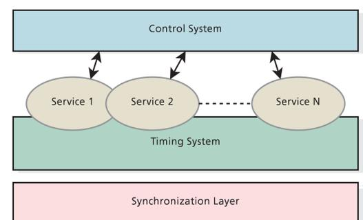
Figure 1: The control system needs several timing critical services, which are provided by the timing system. The timing system itself is constructed on a synchronization layer which provides the basic capabilities to enable implementation of such services.
