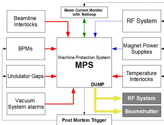
Figure 3: Overview of the MPS system. Red lines indicate alarm signals causing a beam dump. The blue lines are only for analysing the beam losses.
