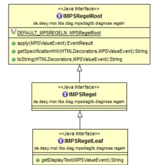
Figure 6: Class diagram of the rule layer
