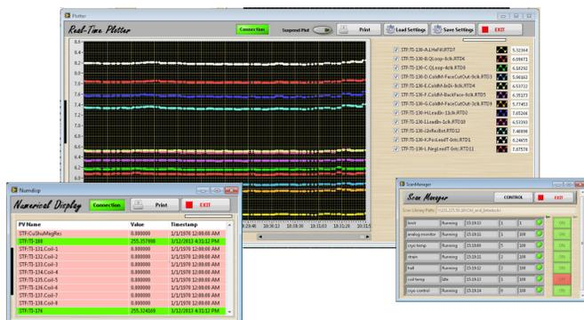
User Interface includes programs for real-time plotting, numerical display and scan control. The plotter and numerical display programs access data through the EPICS CA and can save and restore custom configurations.
