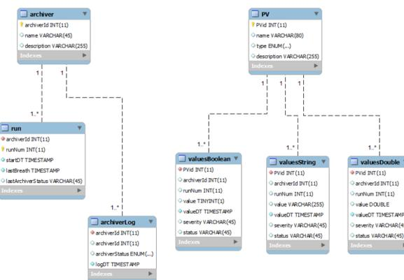
The archive database contains Process Variable data stored as time based information and grouped under runs. A run is defined as a continuous data saving activity of a specific data archiver.
