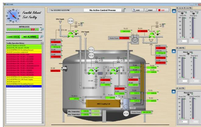
This is the focal UI for systems operation and control. It presents an overview of the system and allows the operator to start automated processes, control valves, and tune and adjust the PID controllers.
