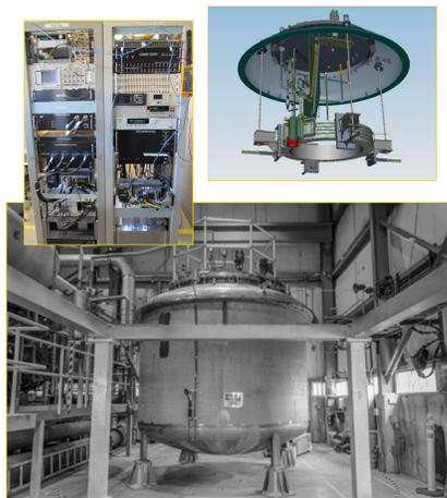
The Solenoid Test Facility is used to test large aperture superconducting solenoid magnets. Its DAQ hardware is based on COTS, such as National Instruments cRIO crates running the VxWorks RTOS and LXI instruments.
