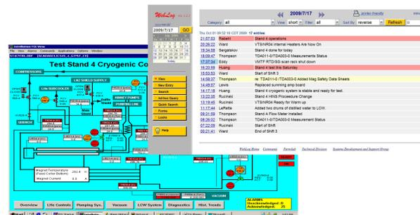
The system interfaces with the IFIX control system for paging, interlocks and alarms. It also makes automatic entries in the electronic logbook.
