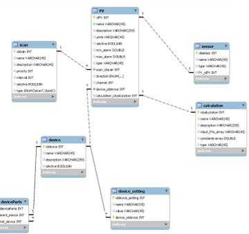
The DAQ and control subsystem is highly configurable. The data model is based on the Process Variable (PV). Each PV is attached to a single device and calculation, and can belong to many different scans.
