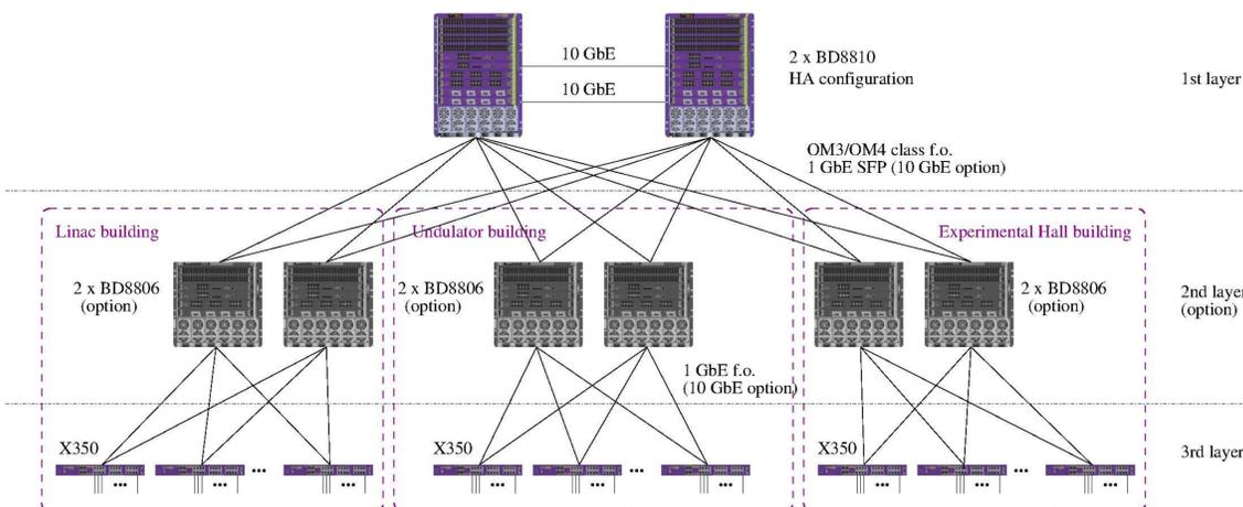
Optical Multi-mode class 3 (OM3) and class 4 (OM4) fiber optic cables, capable of 10 Gb/s (10GbE) network speed over the plant distances, connect the star center, the first and second layer peripheral switches, installed into the controls and diagnostics racks.
