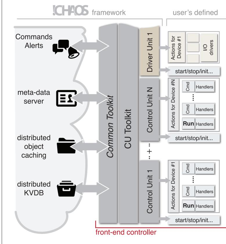
Control Unit is the "container" for a device's front-end controls. Beside the standard methods: INIT, START, STOP and DEINIT, CU specialization is provided by the device's dataset, the actions implemented for it (e.g. commands and control loop) and the drivers for I/O components (see Fig. on the left).
