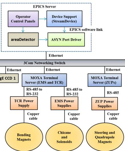
To begin communication with the power supplies and cameras, the synApps software package including ASYN, StreamDevice, and areaDetector was installed.
