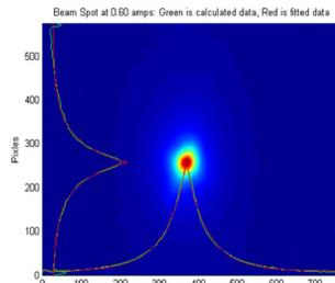
The picture to the right, is a false result from the automatic emittance measurement tool developed by Chris Eckman at Idaho State University.
