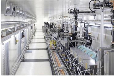
SITF is a highly flexible 250 MeV (~100 m long) linear electron accelerator that has been in operations at PSI for more than three years. The facility consists of a laser driven RF gun, which is followed by an S-band booster section, a bunch compression area and a diagnostics section featuring an RF deflector and a series of FODO cells for the beam emittance control.
