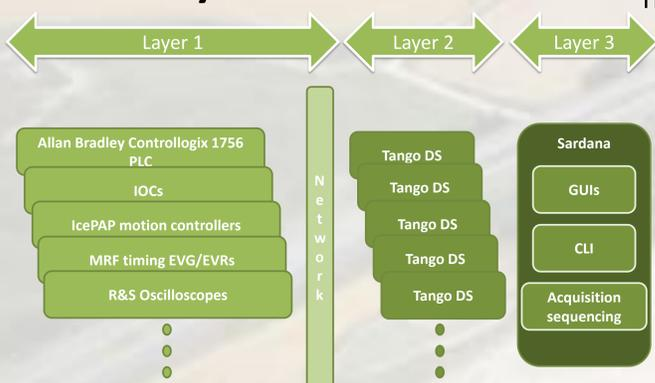
The control system can be split in three levels
