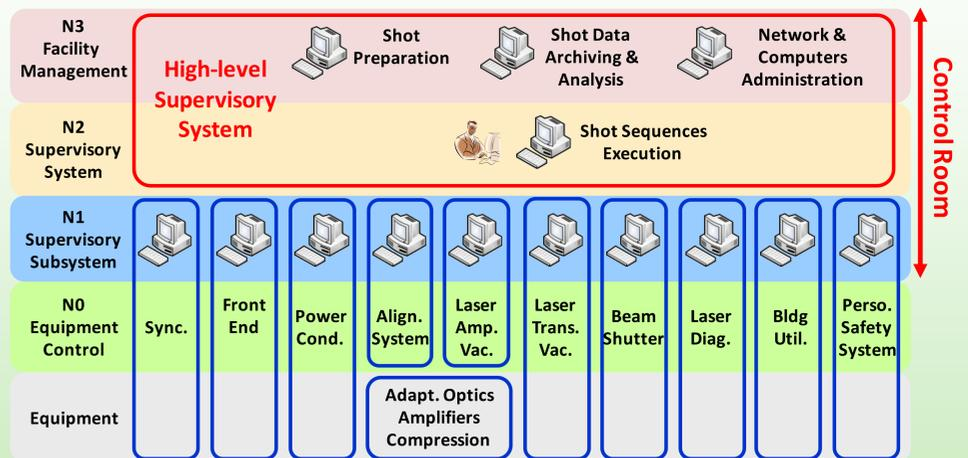
The N1 and N0 layer is divided into 10 major subsystems, corresponding to the main functions of the beam's control system. The Shot Sequences Execution controls the states of each subsystem to lead to the shot.
