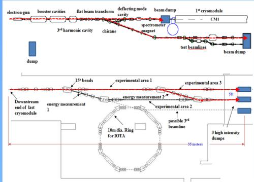
Figure 1 : Machine Layout of ASTA Facility
