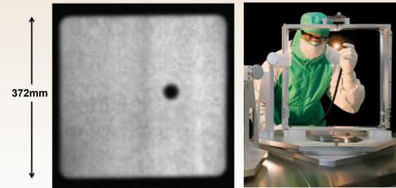
Opaque blockers allow NIF to continue operating even with optic flaws present. This allows optics to be replaced and/or refinished at opportune times during NIF's operational schedule.
