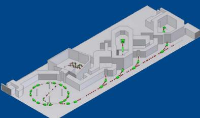
The accelerator, featuring four ion sources, IH-based Linac, synchrotron, three horizontal, one vertical beam line and one proton gantry. Energy ranges from 60 to 800 MeV/u, up to 250 MeV/u proton equivalent for ion therapy [2].
