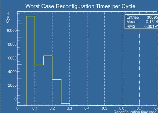
Slowest re-configuration time observed of all PCC application components measured for each cycle.
