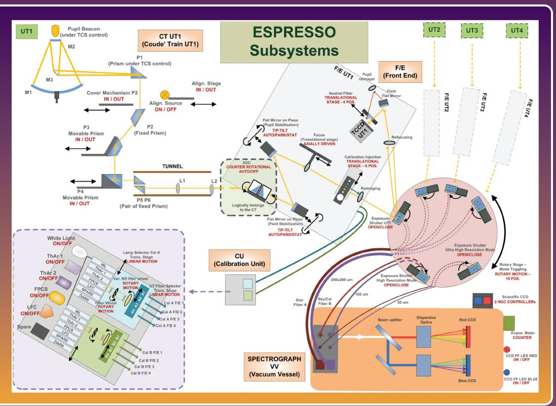
moving parts foreseen in order to maximize the stability and repeatability of the instrument performances. The instrument has two scientific detectors, one for the red arm and one for the blue one. The instrument will cover the whole visible wavelength range (380-780 nm) and its radial velocity precision will reach the 10 cm s<sup>-1</sup> level.
