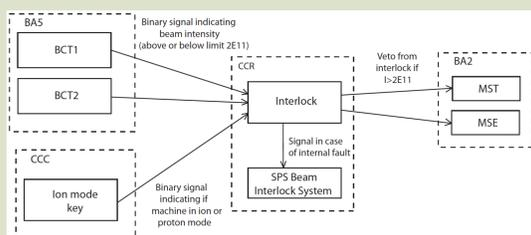
Above: In ion mode two beam current transformers (BCT) at SPS BA5 measure continuously the SPS beam intensity, and if it is above a **set threshold of  $2 \times 10^{11}$  charges**, the interlock maintains a veto on the MSE and MST extraction elements at BA2 to inhibit pulsing.
