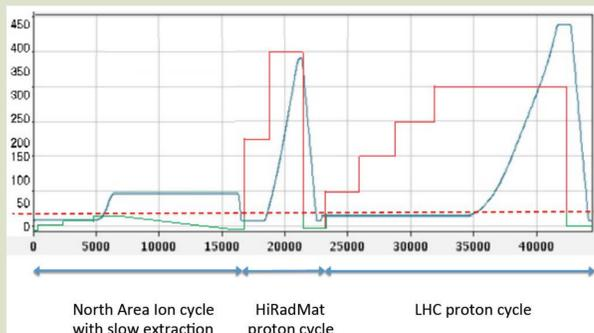
Left: A typical SPS super cycle during a primary ion mode run, comprising a North Area ion cycle at 80 GeV/c/u, a HiRadMat cycle at 400 GeV/c and an LHC cycle at 450 GeV/c. The blue line represents the magnetic rigidity, the green line (red above the  $2 \times 10^{11}$  threshold) the number of charges. The threshold level (dotted line) is exaggerated for the drawing to be readable. The momentum scale is in GeV/c/u, the time scale is in ms.
