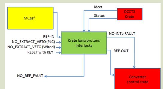
Above: Power converter signal diagram. The reference is sent as an analog signal directly from the SPS power converter control system (Mugef). Interlock signals from both PLC and wired channels are shown as well as the internal safety-check signals from the supplementary DCCT installed
