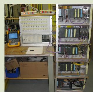
Above: The interlock logic. Delay timers provide a safeguard against a BCT self-check malfunction. MSE/MST internal fault is latched and only resettable with key.
