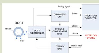
Right: Each DCCT delivers two status signals to the interlock, which indicate the level of beam intensity and the state-of-health of the DCCT.
