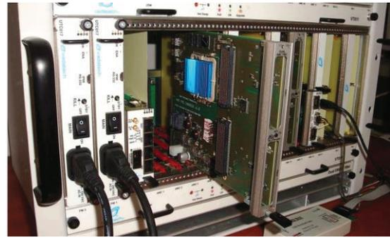
Figure 2: AFC first prototype in a MicroTCA.4 crate.
