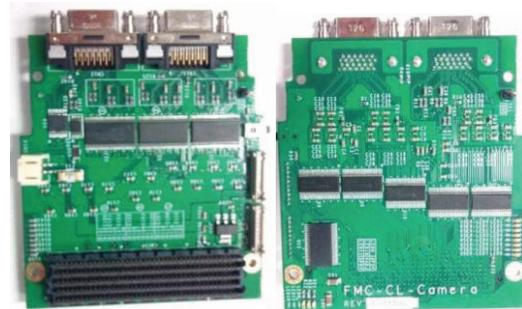
Figure 2: Developed Camera Link FMC.
