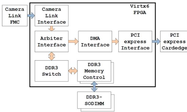
Figure 3: Schematic representation of FPGA logic implementation.
