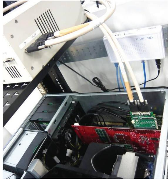
Figure 4: Test bench system for connecting with the interface device of SOPHIAS.
