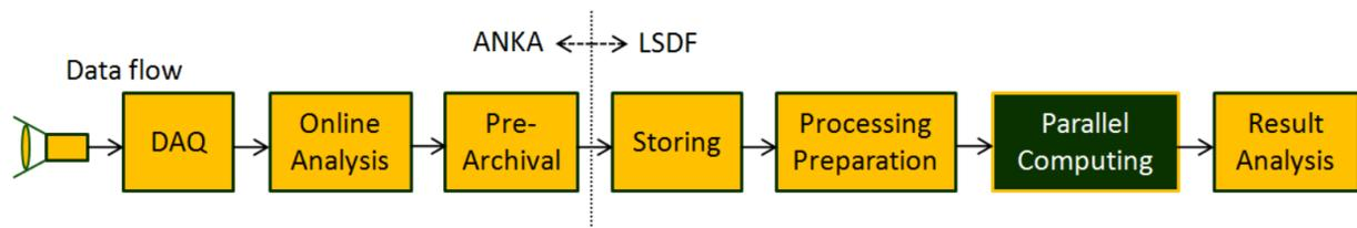
Figure 3: Automatic data processing workflow of LSDF for data analysis of ANKA tomography beamline TOPO-TOMO/IMAGE.
