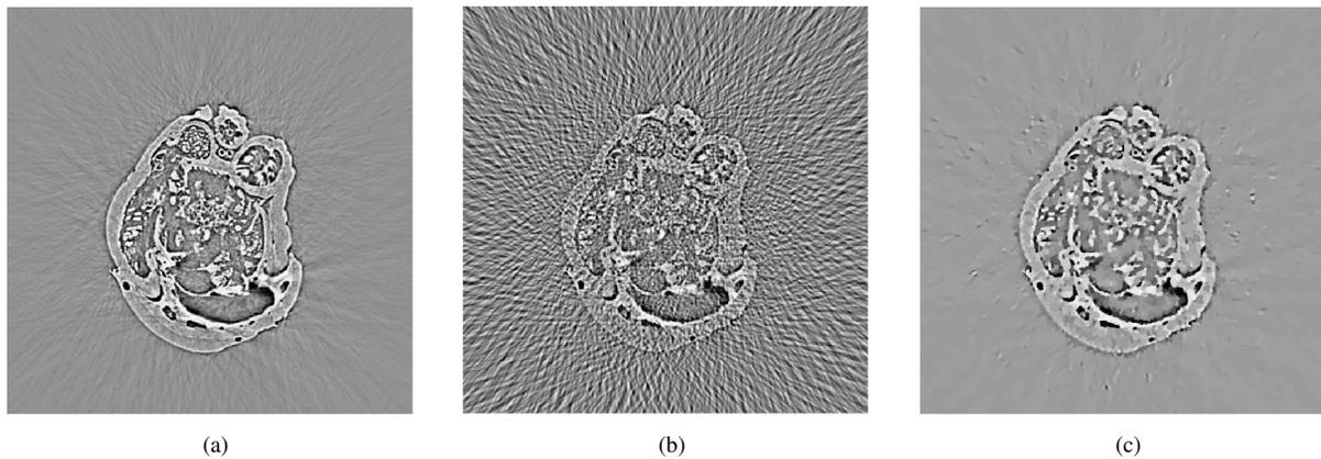
Figure 2: Reconstruction result comparison: (a) is the reference image from 1500 projections constructed by FBP; (b) is reconstructed from the sub-data set, 60 projections, by FBP and shows serious artifacts and streaks; (c) shows the reconstructed image by the CS-based ART method from the same 60 projections.
