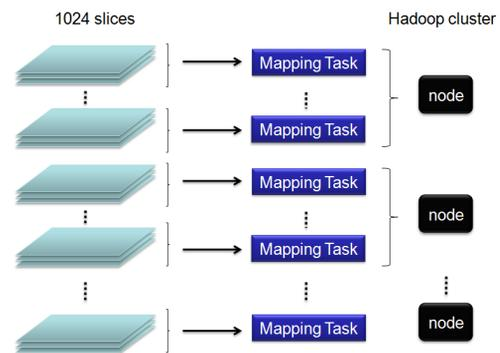
Figure 4: Data parallel computing for 3D computed tomography reconstruction.
