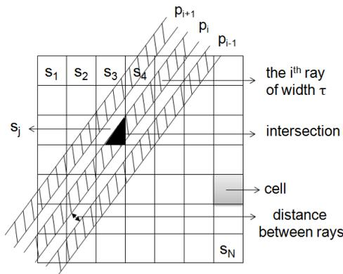
Figure 1: Forward model for ART methods.
