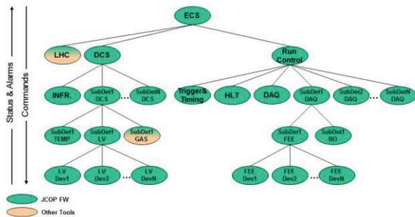
Figure 4: LHCb Control Architecture.
