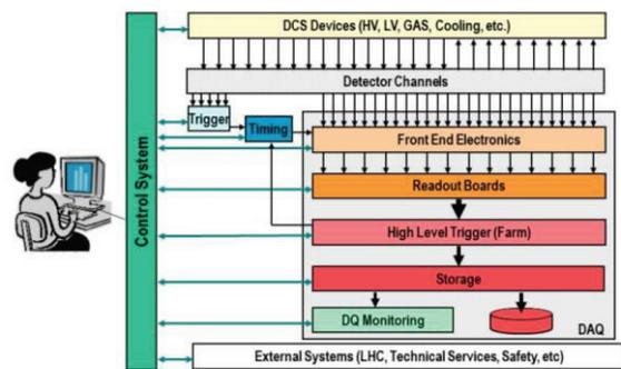
Figure 1. Scope of the Experiment Control System.
