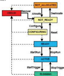
Figure 5: LHCb Run Control FSM.
