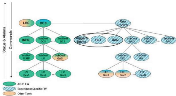
Figure 3: ATLAS Control Architecture.
