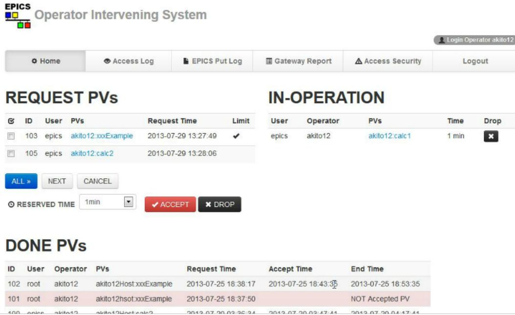
Figure 5: The user interface of the operator intervention system implemented in Ajax.
