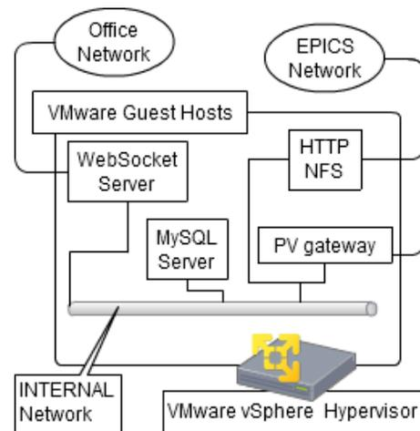
Figure 4: Network chart of the system in the VMware virtualized environment.
