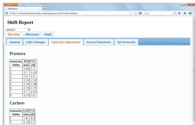
Figure 3: Documentation of changes to the quadrupole settings for several intensity steps.
