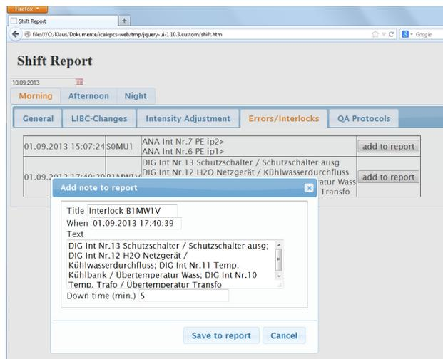
Figure 4: Messages on device failures read from Oracle database. The operator may decide whether they shall become part of the shift report. Error details are automatically included, the operator may add details like accelerator down time.
