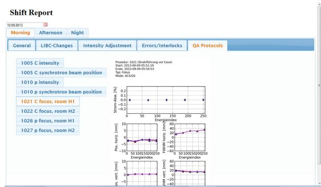
Figure 2: Result of daily QA, like deviation of measured beam intensity from reference values, beam positions and sizes at several places within the accelerator beamlines, and the deviation of the actual currents in dipole magnets from there reference values.
