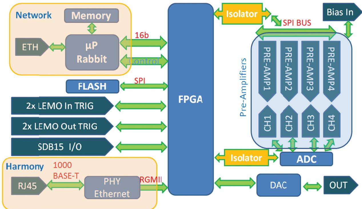
Figure 1: Schema of Alba Em# with the interconnection of the main elements.
